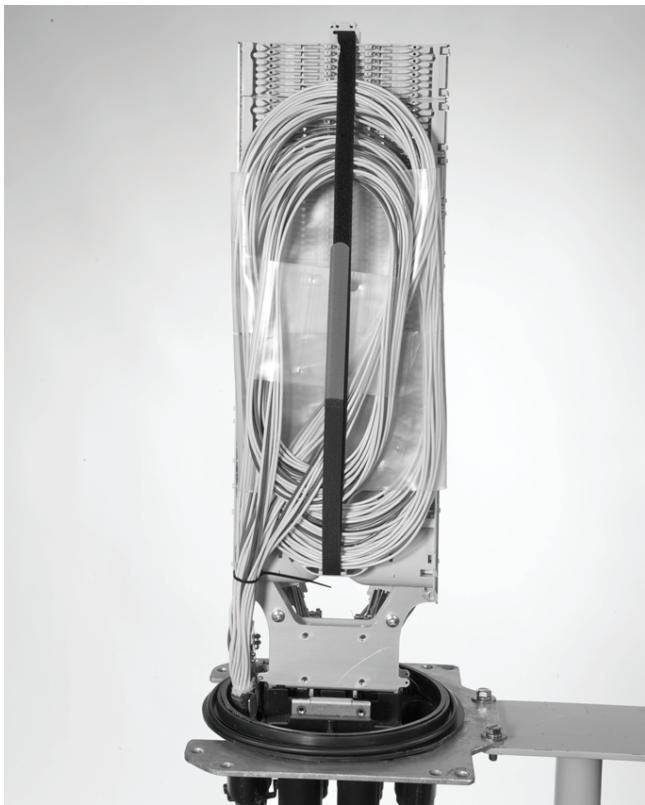
4.1.14 In case a second loop is installed remove the tube holder and store the loop at the unused side of the closure.
