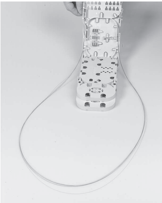
4.1.4 For uncut (shaved) fibers remove jacket accordingly.
