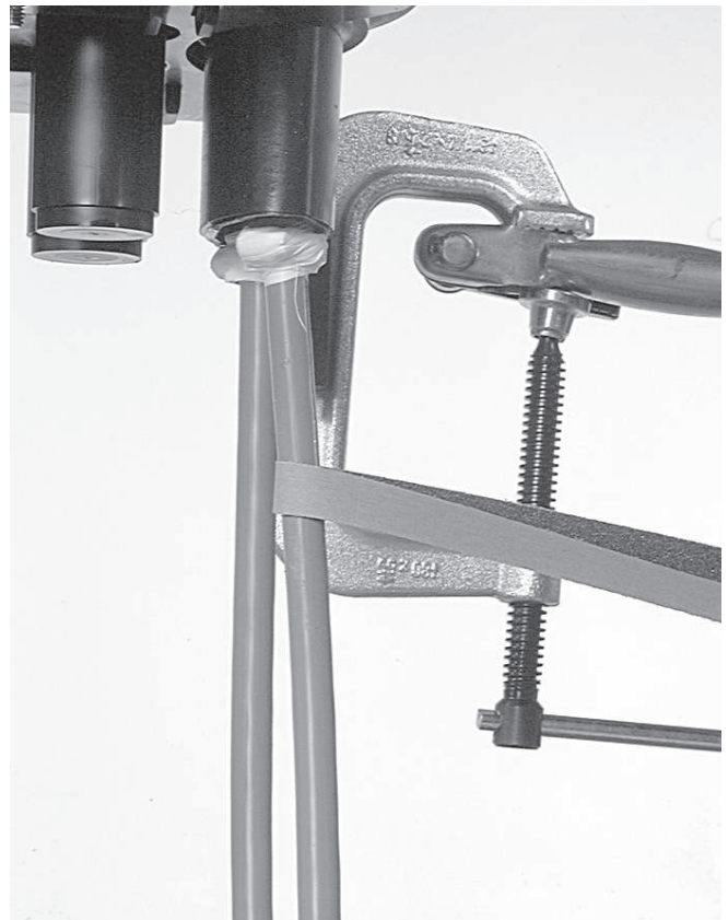
5.1.2 Clean and abrade the cable.
