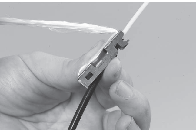
3.4.3 ISROD installation: Put the metal part on top of the cable end, route the aramid strength member over the metal part and make 1 complete turn.
