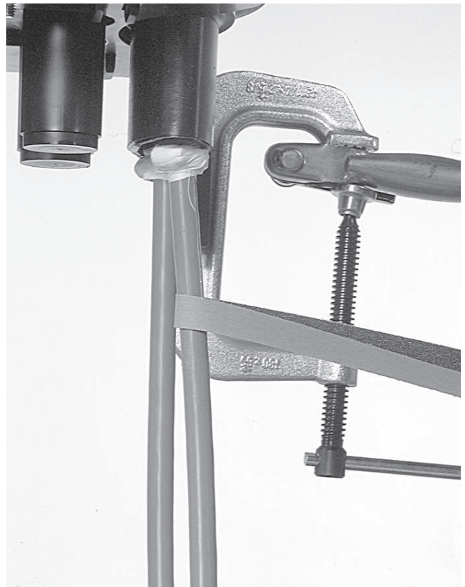
5.1.2 Clean and abrade the cable.
