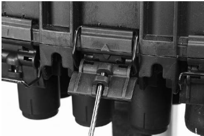
10.2. Closing the latches with a screwdriver.
