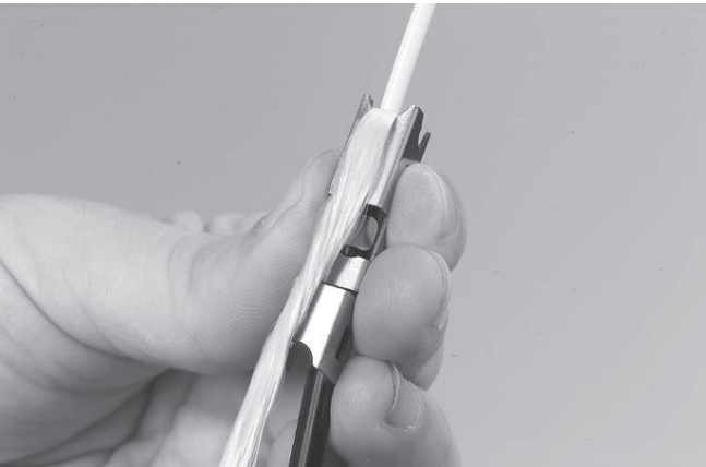
3.4.4 Put the plastic part in the hinge of the metal part and close while holding the aramid strength member under tension (a pair of pliers can be used if needed). Cut the remaining aramid strength member.
