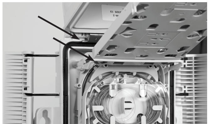
4.1.8 When installation is performed in a vertical position: For lifting the splice tray use plastic wedge. For lifting the cover use metal wedge.
